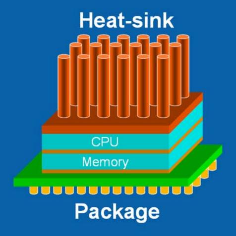
Power and IO signals go through Memory to CPU
