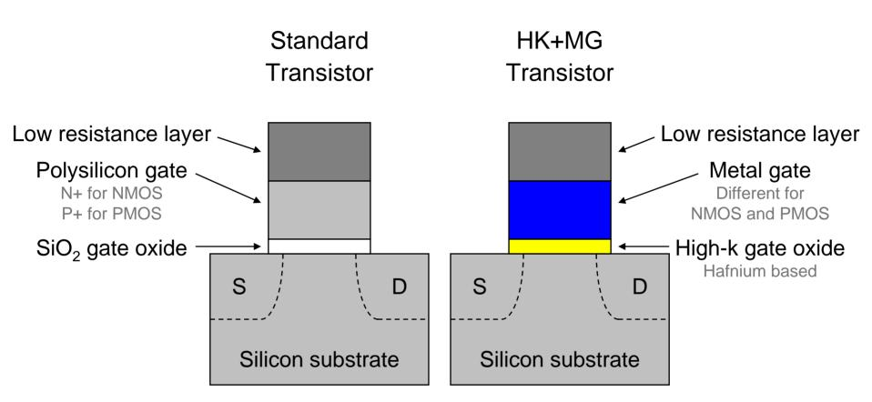
High-k + metal gate transistors provide significant performance increase and leakage reduction, ensuring continuation of Moore's Law
